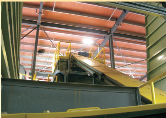
Prefabricated 4 x 400m 3 Quadrant Traverse Silos with Metering Extraction Screws - New Zealand
