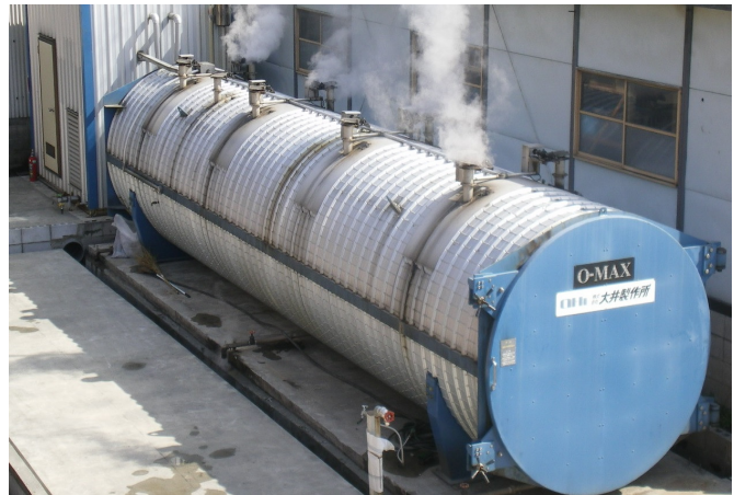
Above: 1 x Cylindrical vacuum drying kiln in Japan.
