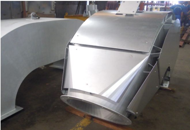
Above: Steel ductings with heat shields.
