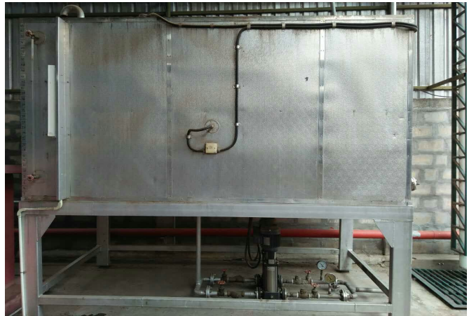
Above: Optional cold water spray system for kilns to replace or assist live steam sprays. Enhances drying quality by limiting kiln over temperatures.
