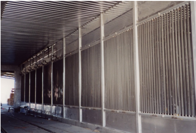
Above: Double track kiln with reheat finned tubes for even kiln drying.
