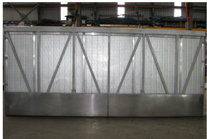
Above: Forklift loaded kiln front panel portal frame structure along with prefabricated panels.
