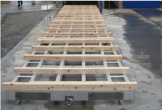
Above: Track loaded kiln bogie trucks shown. Can be aluminum or mild steel. Dual or triple rail.
