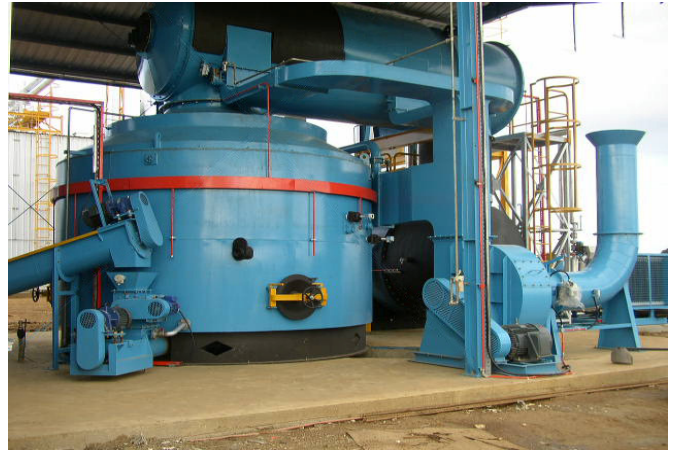
Above: (5MWth) High pressure hot water heater in Australia.
