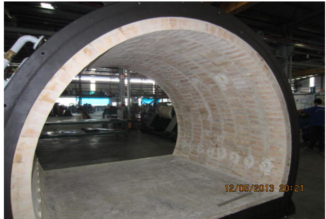
Above: Custom built refractory lined furnace oven for a client.
