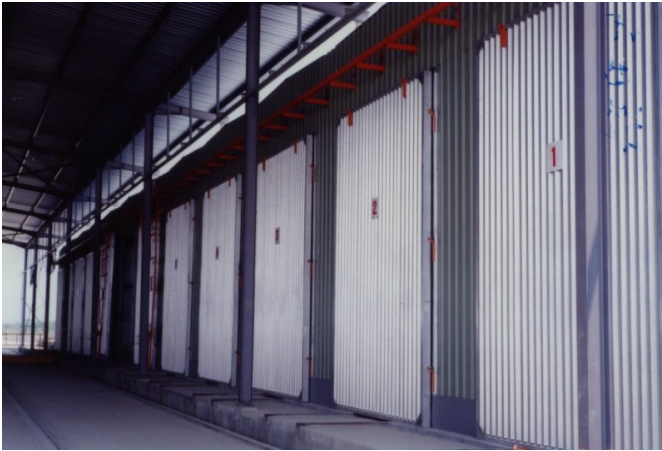
Above: Multiple lift & transfer truck kilns located in a row. (Most suitable setup for this type of kiln)
