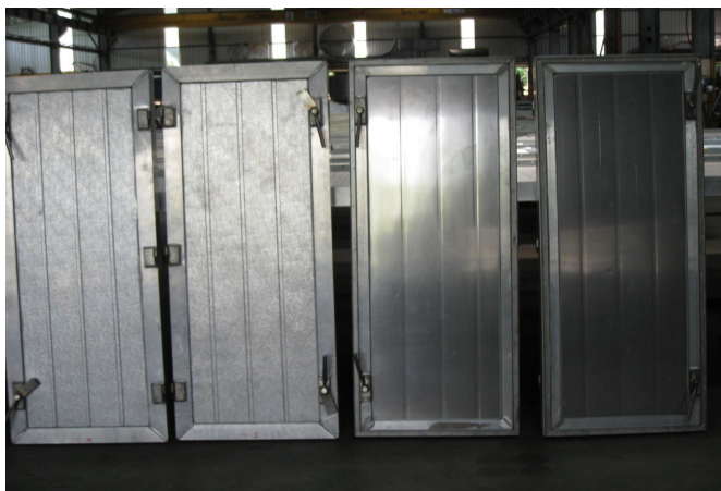
Above: Sample kiln inspection door panels made out of rigid polyurethane insulation. Wrapped in a aluminum extruded frame and sheathed (inside = stainless, outside = aluminum) sheets.
