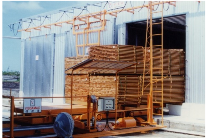
Above: Lift & transfer truck system loading timbers into a conventional truck loaded kiln.
