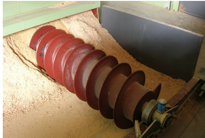
Above: Silo metering discharge screw.
